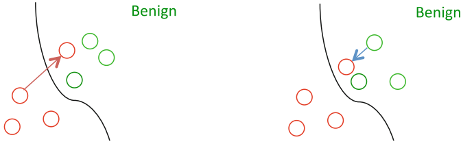
Fig. 2. A simplified example of the mimicry and reverse mimicry attacks. On the left (mimicry) it can be seen that the features of a malicious sample are changed to go into the benign region. On the right (reverse mimicry) a benign sample is injected with malicious content with few structural changes, so that the sample could keep staying in the benign region.
