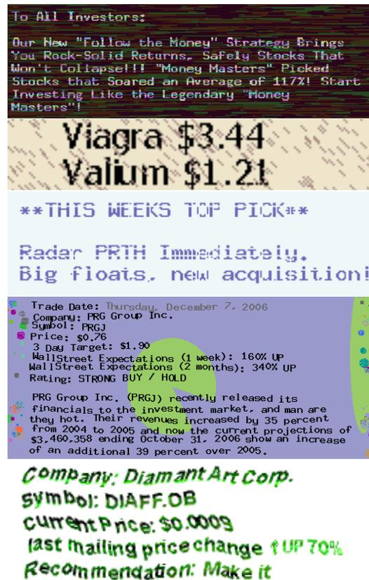
Figure 7: Examples of real spam images (details) from the data set used for the experiments, with different kinds of content obscuring techniques. From top: multi-coloured text interfering with non-uniform background; small random noise interfering with text; characters broken by lines of the same colour as the background; non-uniform background; a CAPTCHA-like technique.
