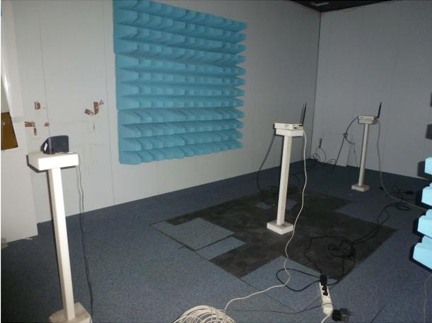
Fig. 4. Image of the test bed used to collect the radio frequency emissions
