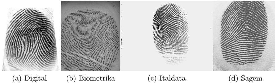
Fig. 2. Examples of fake fingerprint acquired with the 4 sensors
