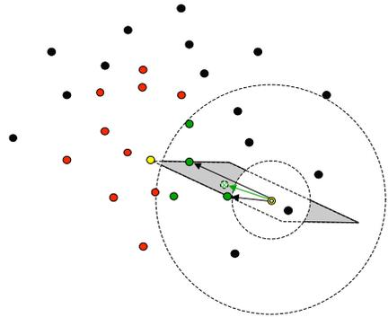
**Fig. 1.** Example of *K-NN* “synthetic” pattern generation in a two-dimensional feature space, where  $K = 2$ ,  $\xi_1 = \xi_2 = 0.5$  and  $\lambda = 1$ .
