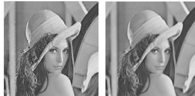
Lena image watermarked with q = 47\text{dB} (left) and unmarked with M(q) = 37.37\text{ dB} (right).
